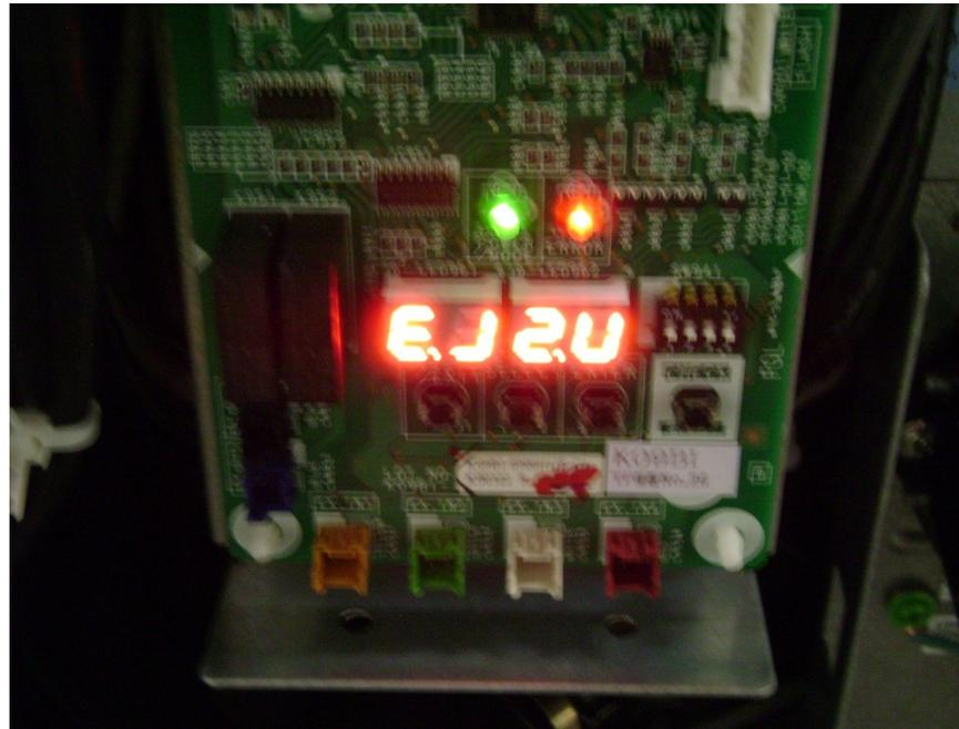
To begin, inspect all branch boxes for anything other than a solid green LED on LED402. With the *EJ2U* error code, it is not uncommon to see the following error codes registered on the effected branch box:
