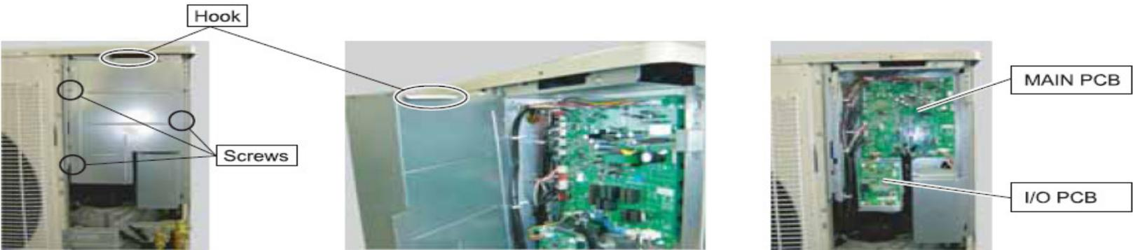
The first image shows the front cover being slid towards the left, with callouts for 'Hook' at the top and 'Screws' at the bottom. The second image shows the front cover removed, with a callout for 'Hook' at the top edge. The third image shows the internal components, with callouts for 'MAIN PCB' and 'I/O PCB'.
